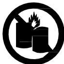
Do not place flammable objects (cloths, curtains, etc.) on or against the stove. Do not cover it under any circumstances or move it while it is in operation. Do not store chemicals or flammable materials near it.
